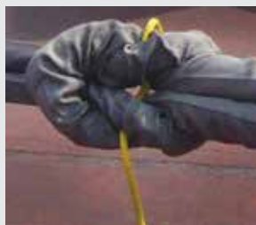
Cow hitch connection, shown with pigtails to assist in separating the connection.
