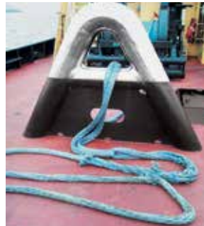
Single-leg pendant-to-mainline connection.
