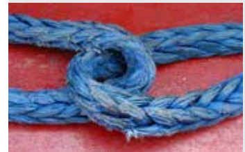
AmSteel®Blue mainline with eye-to-eye connection to AmSteel®Blue pendant.
