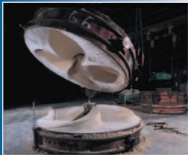
The use of "no bake" sand in molding Federal Propeller patterns result in extremely accurate castings.
