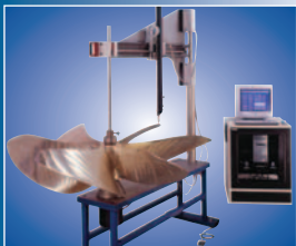
Sophisticated measurement recording instruments (Hale MRI) facilitate full documentation and perpetual record.
