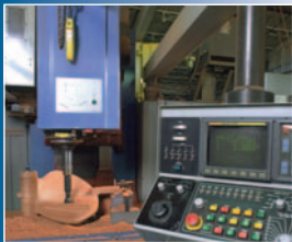
All patterns are machined cut on computer driven CNC cutting mills. This assures that the design criteria will carry through to the propeller castings.
