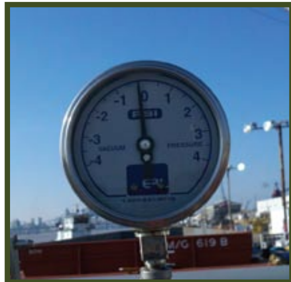
Model 505 stainless steel Pressure/Vacuum Gauge mounted on Vapor Header.
